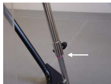
Fig 6: The mark indicating how far the support leg should be drawn out to get an inclination-angle of 5^{\circ} .
